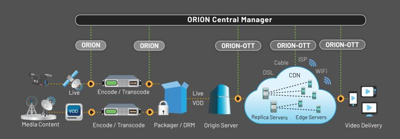
ORION-OTT monitors ABR content, both VOD and live, using user-defined automated / manual schedules. It checks for inconsistencies pertaining to ABR package compliance, manifest / playlist syntax, download errors, content quality and more. It can also be used for origin server load testing.
